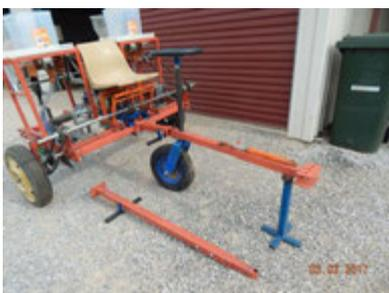
This is an optional arrangement to lessen turning circle. The drawbar is hinged along its length with the front section rigidly attached to 2WT. It also has the tailwheel fitted. The tailwheel is steered by the operator. The tailwheel can be re-configured as per the pictures of the mounted model shown below.
