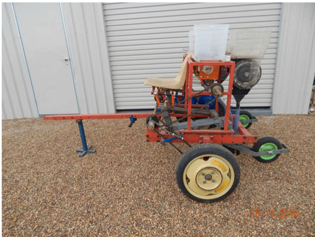
Experimental two row trailing planter for two wheel tractor.
