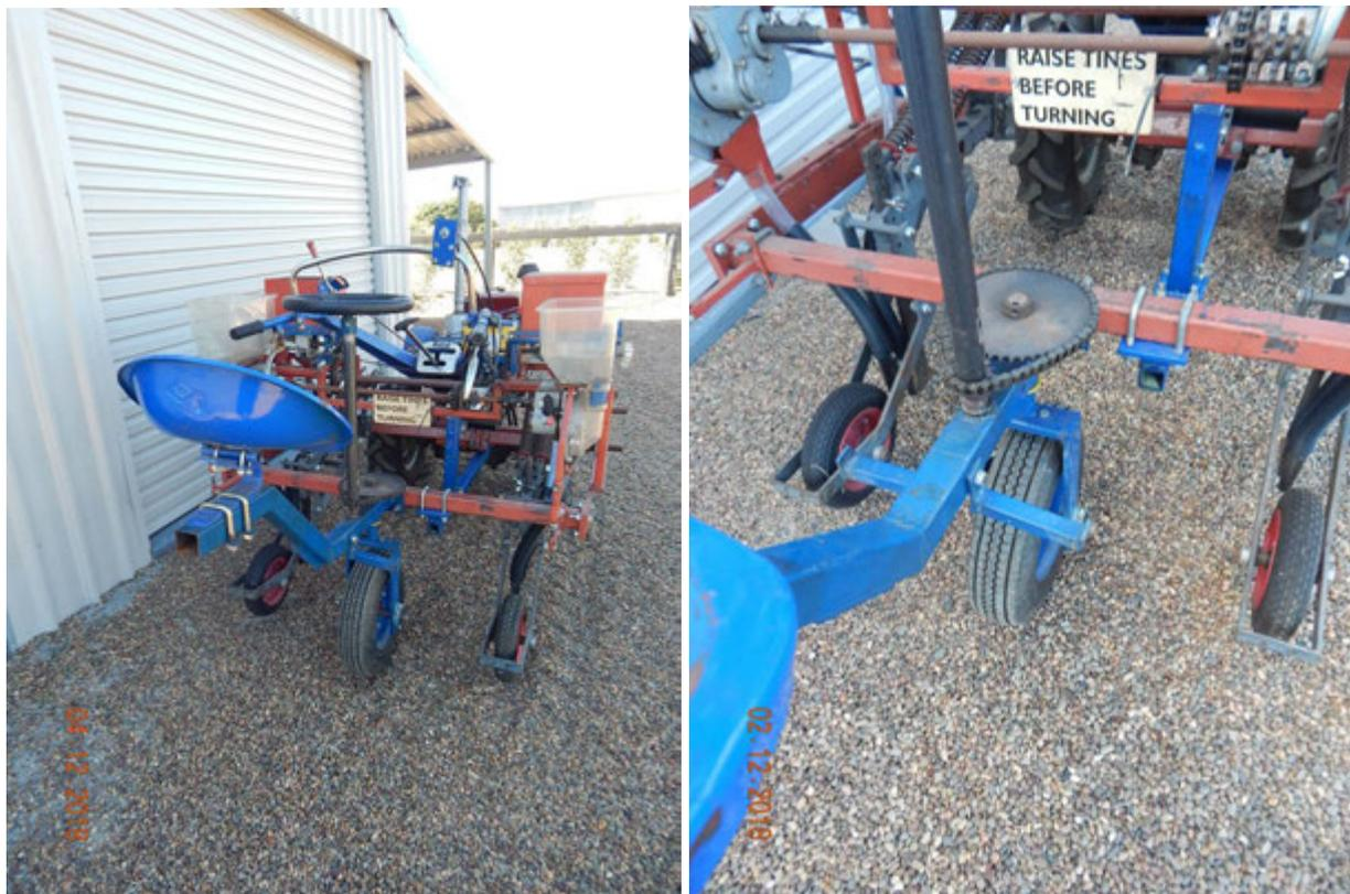
In my initial operation of the Gongli Africa 3 with a standard tail wheel I found it completely unsatisfactory. It was nigh impossible to steer with your feet, as too much effort was required. In addition, with the castoring tail wheel reversing was dangerous. Upon reversing, the castor wheel attempted to spin through 180 degrees, and could cause severe foot damage when attempting to steer by this method.
