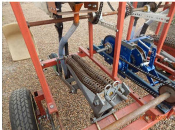
Spring loaded tine assembly (spring compression adjustable)
