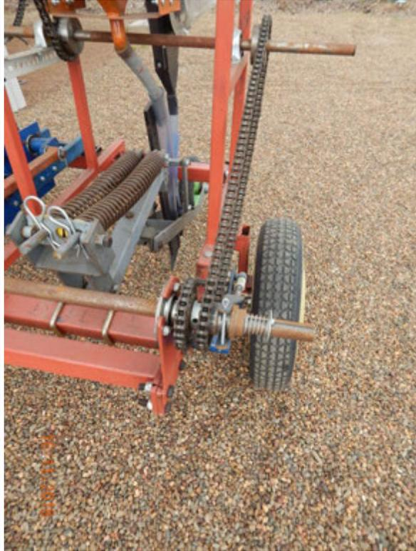
Mechanical lift assembly- it is under the operator seat which has been removed for the picture
