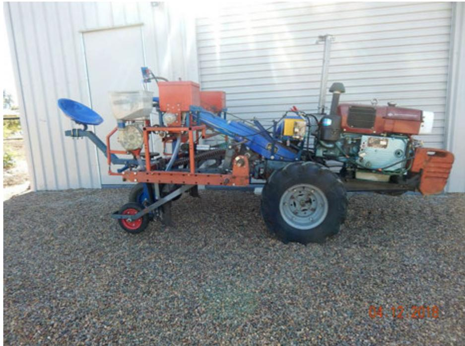
This unit has undergone several more modifications since the initial report last year. First, it now has a 12 volt linear actuator with a stroke of 100mm and a capacity of 200 Kg to do all the lifting and lowering. However this option is only available if the tractor has an electric start with a battery.
