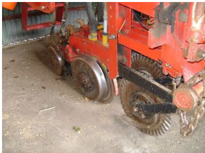
Bertini planting line which comprises a fluted roller for residue cutting, off-set twin disc openers for seed and inclined seed covering wheels. The machine has an additional hopper for slug pellet application
