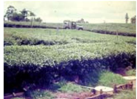
One end of the site, at full canopy, after the end of the trial, also showing the drums used to catch soil and water from each individual plot.
