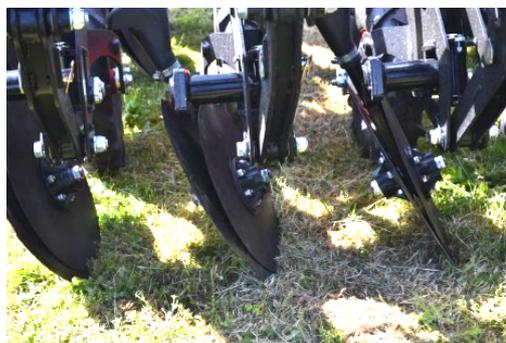
Figure 4. Inclined double offset disc openers on the Weaving drill
