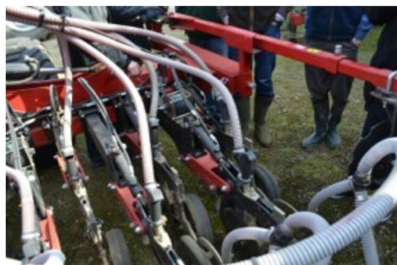
**Figures 3 & 4. Weaving Big Disc zero-till seed hopper with pneumatic fan; on the right the planting line with disc openers for seed. The drill costs around £50,000**
