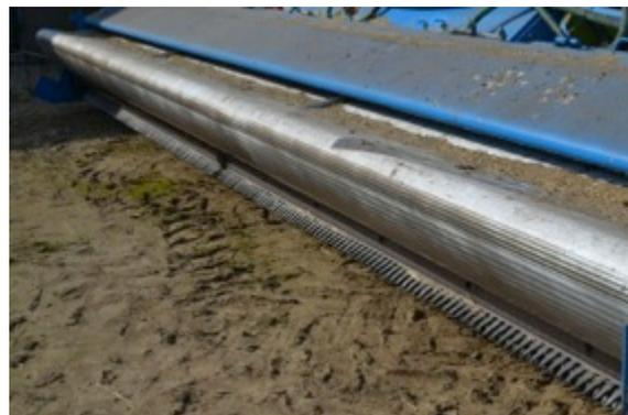
**Figure 5 Shelbourne Reynolds Combine and 'stripper head'**
